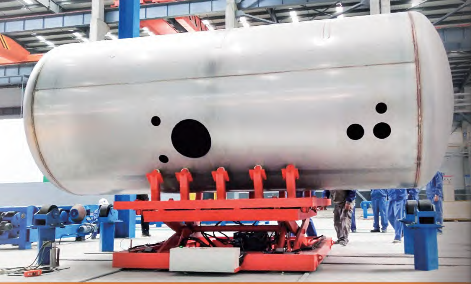
But this series have strict requirement on the construction of the railways which need to be insulated. The rated load can not be more than 50T.
